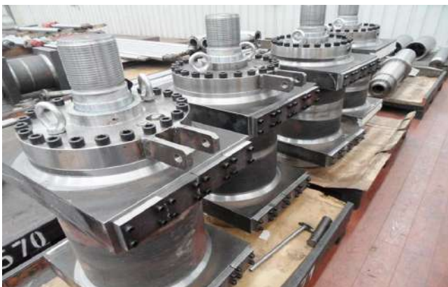
Hydraulic Cylinder - Cement Plant
